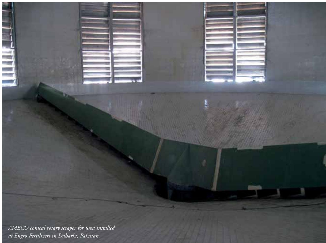
*AMECO conical rotary scraper for urea installed at Engro Fertilizers in Daharki, Pakistan.*
